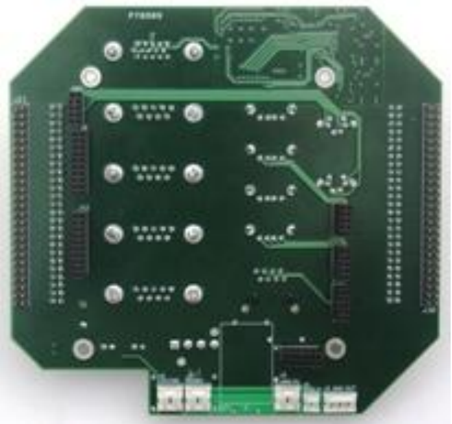
Aurora Panel I/O Board, SBC Side
